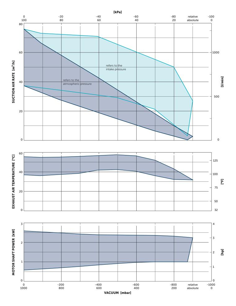
Reference data (atmosphere): 1000 mbar (100 kPa), 20°C (68°F) Tolerance:  $\pm 5\%$
