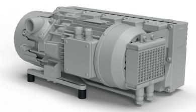
U 5.40 XL K with a 1,0 Liter oil tank, an oil-air cooler, a gas ballast valve, a suction connection that can be rotated in 90° steps and a threaded connection for the exhaust air.
